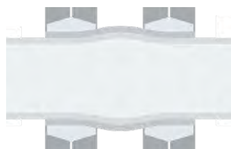
Pressed Condition (cross section)
