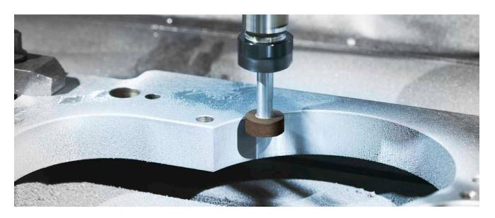
These polishing points are available in one grit combination only. The surface finish is similar to a finish with grit size 100. The hard rubber bond makes these points particularly suita-
