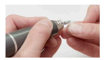
LUKAS polishing points, wheels and lenses are specially designed for fine mechanics and laboratory work. But with their soft elastomer bonding, these tools are also a valuable aid in other areas such as pattern construction or jewellery. Available in tiny sizes and a wide range of shapes, they make it possible to machine even the finest workpieces and textures.
