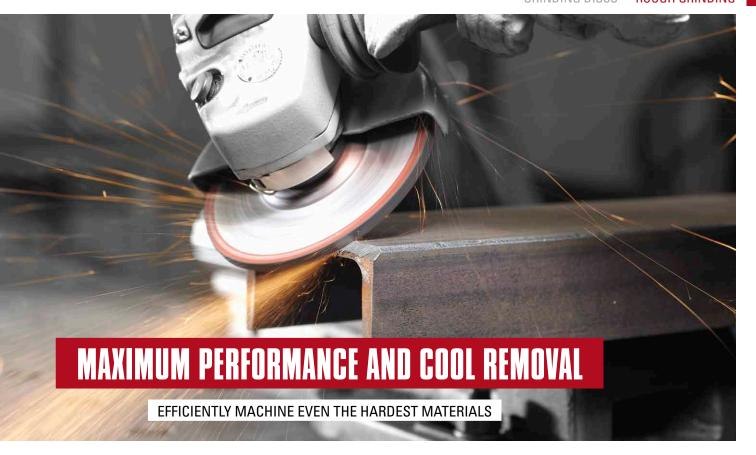
The LUKAS grinding discs with ceramic grain are perfectly suited for highly productive machining of steels. Thanks to the fast but cool cutting, they can machine inox without any blue discolouration and have an exceptional tool life due to the self-sharpening effect. In addition, these require only little effort during use. The low applied grinding pressure also contributes to low operating temperatures.
