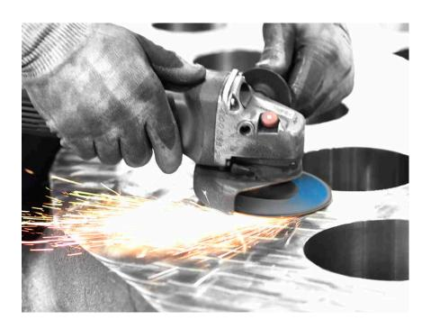
LUKAS NAWAROFLEX® lamellar flap discs have a backing plate made of renewable raw materials. Although made of paper, these special eco-friendly backing plates are nevertheless very sturdy and offer enough stability for hard grinding applications.
