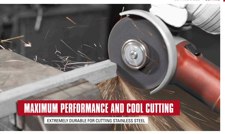
LUKAS cutting discs with ceramic grain are perfectly suited for high performance steel cutting. Thanks to the fast but cool cutting, they can machine inox without any blue discolouration whatsoever and have an exceptional tool life due to the self-sharpening effect. In addition, this tool requires little force to be applied.
