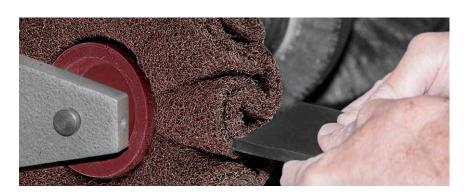
LUKAS mops of abrasive fleece are packed together on a shaft to create rolls of different widths. By adding water or low-viscosity oil, you can further boost the service life of this tool: Water produces matt surfaces on almost all metals and very matt surfaces on aluminium, while oils give a silky lustre finish.
