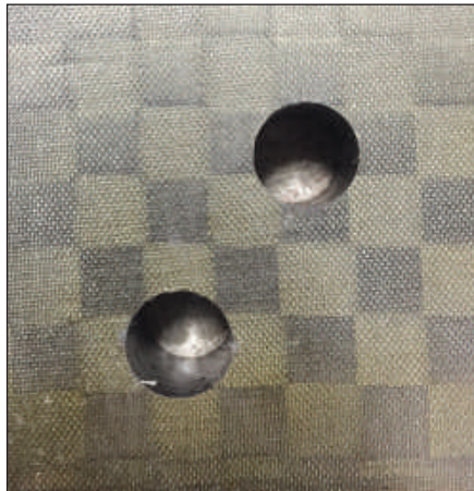
Holes drilled with PCD tooling
