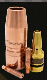
This system features our well-known TOUGH LOCK® Contact Tips and Retaining Heads. TOUGH LOCK Contact Tips are precision-machined using a process that tightly controls tip tolerances. TOUGH LOCK Retaining Heads are manufactured with a tapered design at both ends that keep the consumables locked from tip to neck for improved weld consistency and to maximize heat dissipation.
