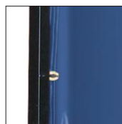
Brass grommets & nylon ties secure welding curtain to frame
