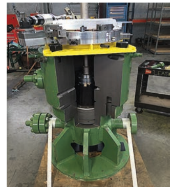
EICC Casing Cutter used for wellhead completion
