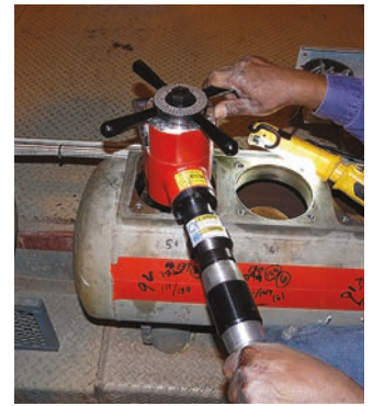
Box header beveling with SDB
