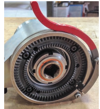
Fast, tool-free drive motor mounting
