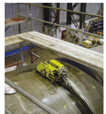
Trav-L-Cutter being used for submarine decommissioning
