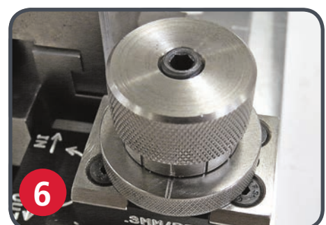
6 Rapid Adjust and Micro Adjust knobs provide greater precision during setup & operation
