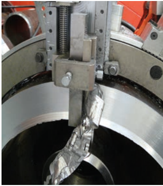
DynaPrep MDSF enhanced form tool capabilities
