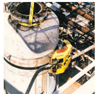
Add mounting chain sections to fit larger diameters
