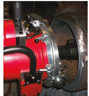
Self-centering standard mandrel
