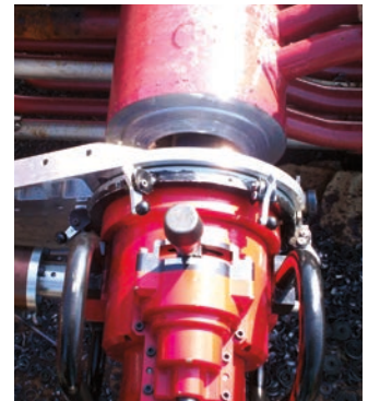
EP 424 single pointing deluxe prepping heavy wall pipe
