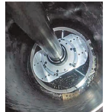
Internal cutting module lowered to cutting depth
