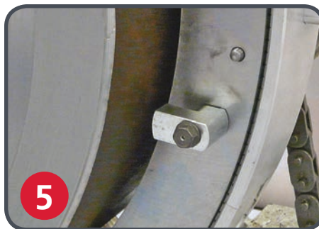
5 Captivated, swing-away toe clamp for easier slide mounting
