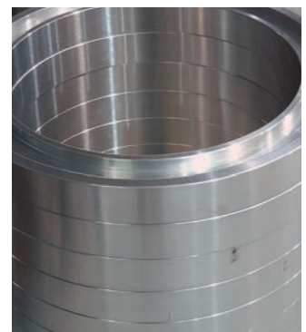
Machined split frame rings
