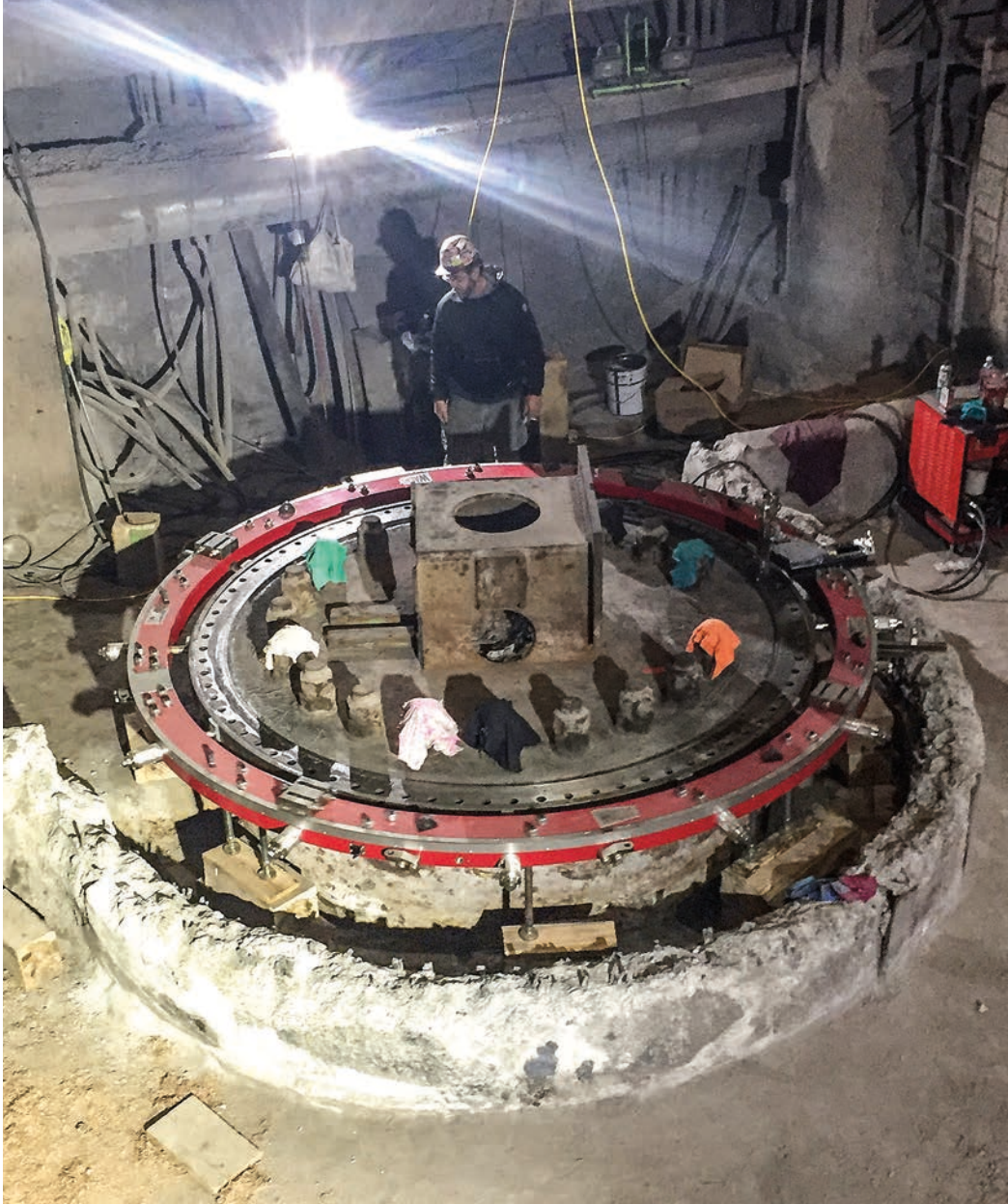
LDSF splits into quadrants for setup, transport & storage
