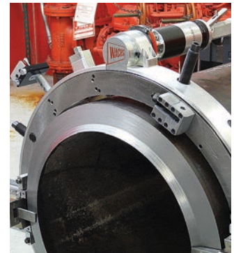
Powerful air motors for greater form tooling capability.
