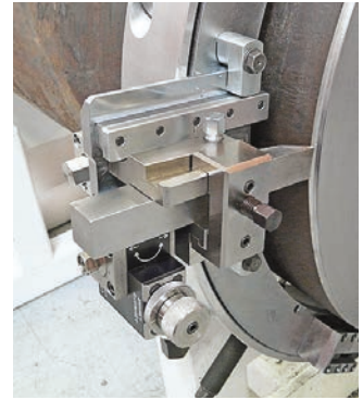
Slides feature Rapid Adjust and Micro Adjust
