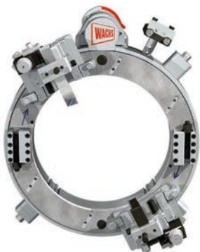
Split frame bolted together
