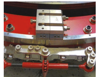
Swing bolts & hinge mechanism speeds assembly & mounting
