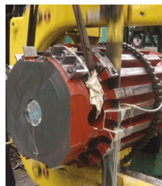
Guillotine Goliath cutting powerplant turbine shaft
