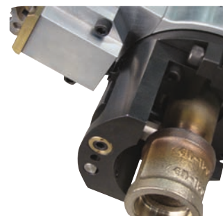
Axial Slide for Socket Weld Removal
