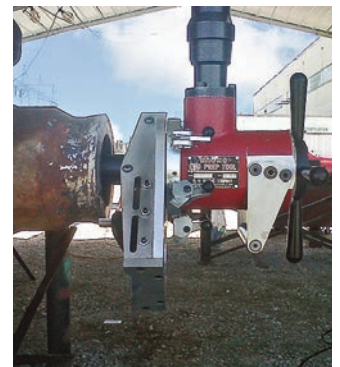
SDB end prepping pressure vessel
