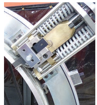
OD tracking slides follow out-of-round pipe & vessels.
