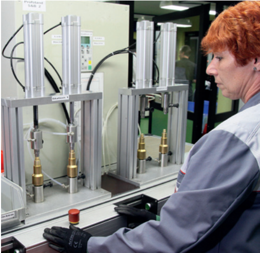
AUTOMATIC TESTING EQUIPMENT FOR GAS RETURN, LEAKAGE AND FLASHBACK TEST
