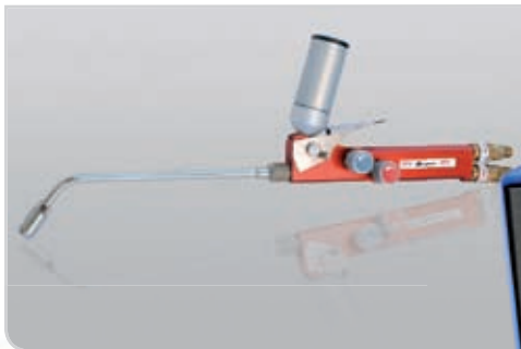
Tip 550mm with Tungsten Carbide inserts
