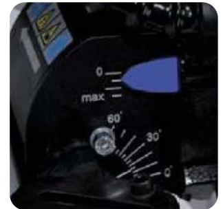
Continuous angle adjustment from 0 to 60 degrees.
