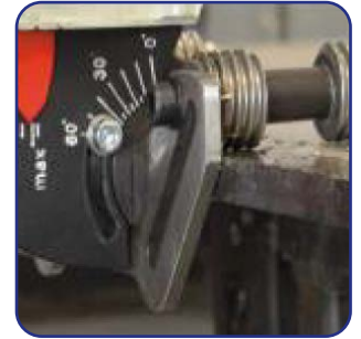
Continuous angle adjustment from 0 to 60 degrees.
