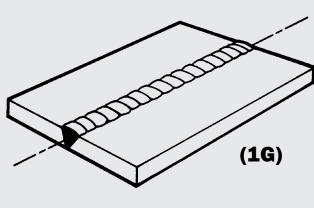
Plates and Axis of Pipe-Horizontal
