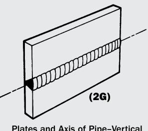
Plates and Axis of Pipe-Vertical
